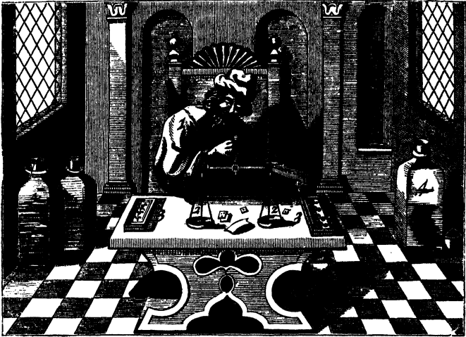
Fig. 129. 1. Assayer. 2. The scales. 3. The cases for weights. 4. Glasses for aqua regia, aqua fortis, aqua vitrioli, aqua argentum, and quicksilver. (Pettus.)
